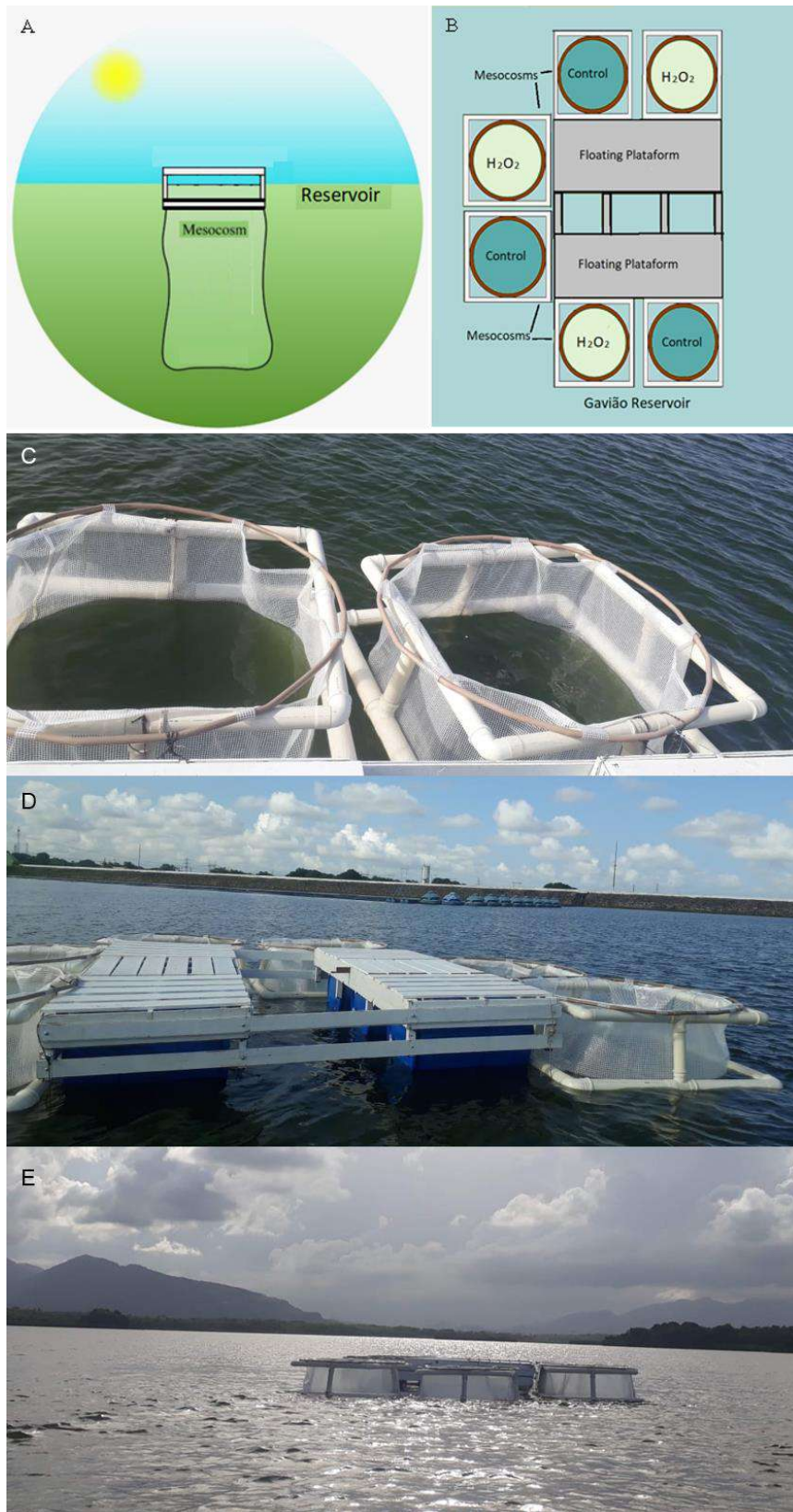
Figure 1: Design of experimental platform, using illustration of individual mesocosms (A), the floating platform in top view (B) and real photographs of structure assembled in the Gavião reservoir (C, D and E).
